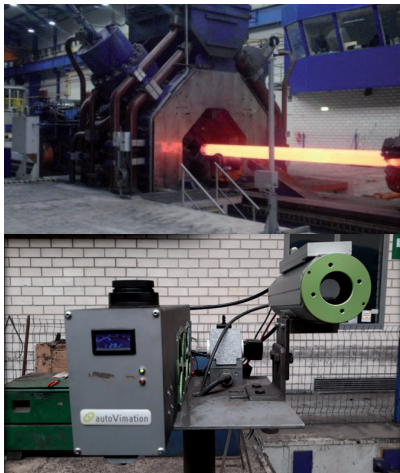
Figure 4: Shows a photograph of the forging machine and the enclosed camera equipped with a cooling system.
