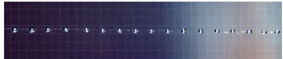
Figure 4: Experimental visualization of jet breakup at a vibration frequency of 220 Hz and amplitude of 100 \mu\text{m} , with a liquid column height of 280 mm (grid spacing – 4 mm)
