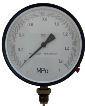
Figure 1: Verification pressure gauge.
