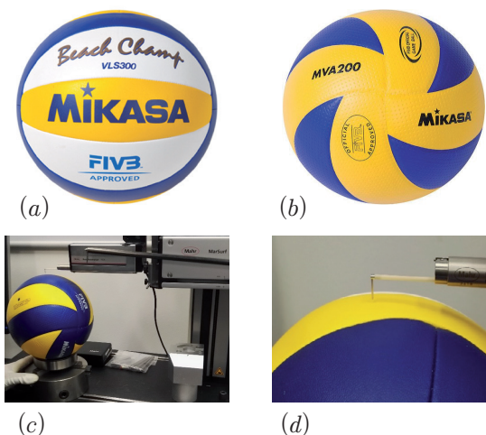
Fig. 2: (a) Beach Volleyball Mikasa VLS 300. (b) Volleyball Mikasa MVA 200. (c) Setting of the ball and sliding unit of measuring machine to the position. (d) Probe position on the surface of the volleyball.
